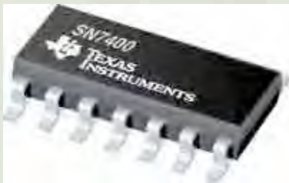
Texas Instruments, SN7400, 8 transistors, 1966
